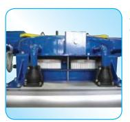
Integrated reverse air jet-cleaned dust filtration and reclaiming system (dust collected is re-introduced into the chute).
