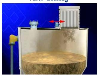
Dust drops down into the silo due to shaking filter elements
