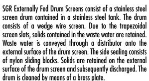
After passing through the inside of the drum screen, clean water is collected on the bottom of the tank and discharged through a nozzle. Rotation of the filter occurs by coupling connection to a gear reducer mounted at the end of the drum. At the opposite end a cleaning system is installed. The system is composed of a pipe equipped with a high pressure nozzle which periodically cleans the filtering drum (mobile washing system). The system has to be connected to the water mains.
