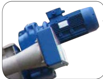
Single drive unit for drum and conveyor screw
