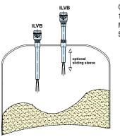
G1½" ISO 228 or 1½" NPT ANSI B 1.20.1 Material: 304 SS Sealing material to the extension tube: NBR
