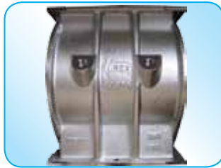
Lateral air venting bores as standard Used for: - extracting excess air from rotor pockets - decreasing air pressure inside the casing - increasing throughput
