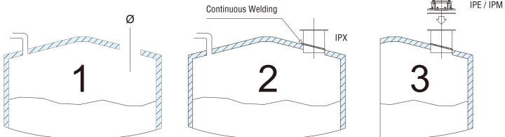
Commonly installed on the roof of the silo or container, IPE and IPM are used to monitor the pressure level inside the silo or container.
