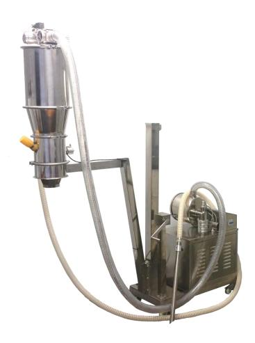
Capable of transferring up to 800L/hr of product, the FVC-1 can handle most small factory needs. If a higher transfer rate is required, please ask us about the bigger brothers of the FVC-1.
