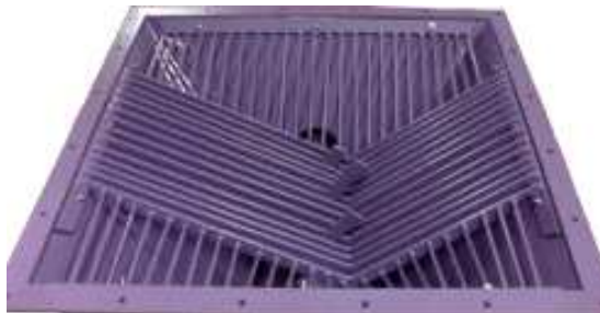
Lump breaker system in a hopper of a big bag unloading station.
