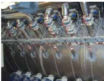
Choppers, liquid injectors, temperature jacket
