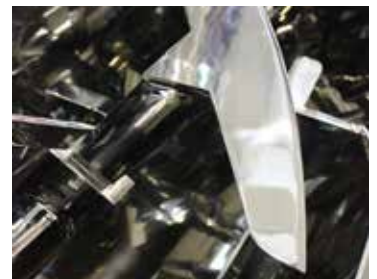
304L / 316L stainless steel internal polishing
