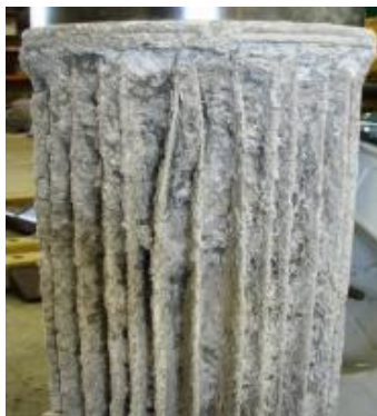
Vac Truck Filter that has not been maintained
