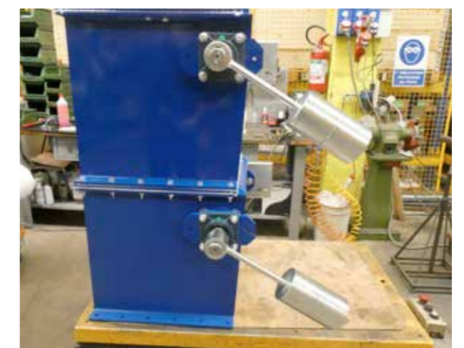
COUNTERWEIGHT VALVE: in this case, the activation of the flaps depends on the weight of the material.
